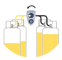
When the empty cylinder is changed, the person who exchanges the cylinder will then turn the Clesse indicator knob to the existing part-used cylinder ready to indicate when it becomes empty – this then becomes the "Service"
